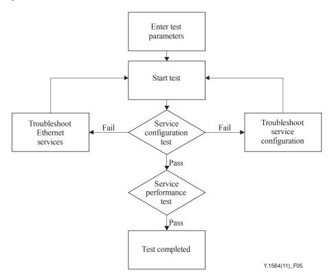
Figure 5 – High-level service activation test methodology
