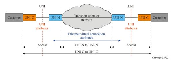
Figure 2 – Single provider view of Ethernet service areas
